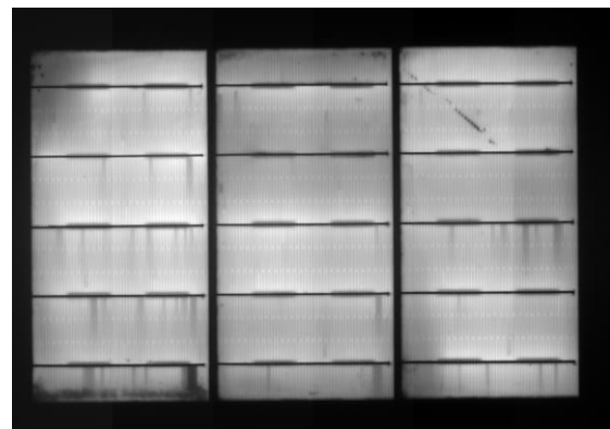
(c) EL image of PV module E-1 after the combined test UV-DH (120 kWh/m 2 ) followed by TC 200.
