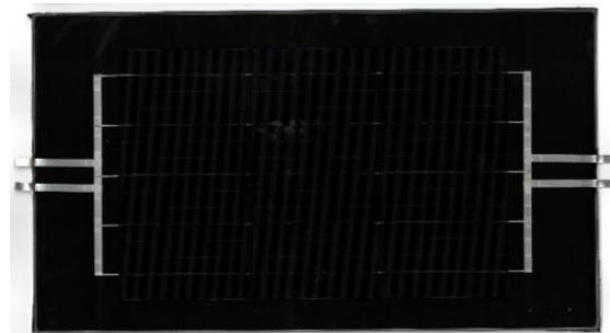
(b) Photograph of PV module E-1 after the combined test UV-DH (120 kWh/m 2 ) followed by TC 200.
